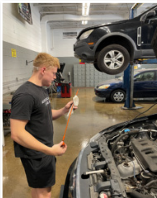
Photo: Cameron checks the engine oil level and color during his vehicle maintenance unit.
