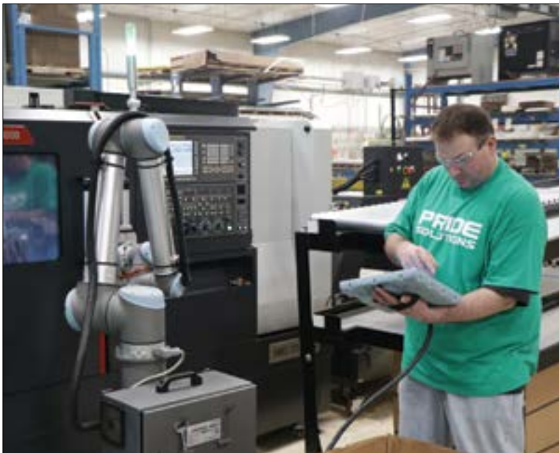
Pride Solutions in Hutchinson took on a project to automate their CNC with a collaborative robot. This machine operator learned to program the Universal Robot during the project. Credit: Pride Solutions, Hutchinson, MN
